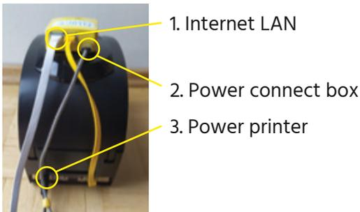
**2** Push the "Power" button to turn on the printer and wait a few minutes. **Check that all LEDs on the yellow box are on (except for the "status" LED that blinks every 3 seconds).**
